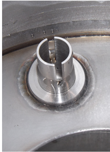
Figure 4.17. Photo of the leveling bellow in the TPC-vessel. The vessel is filled with water to test the surface tension effect on the gaps.
