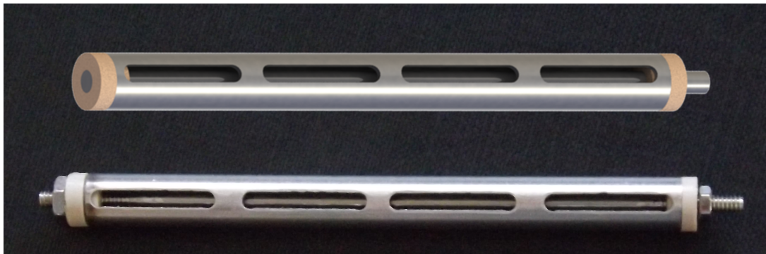
Figure 4.14. The levelmeter of the buffer volume. On top the rendered CAD-version, on bottom a photograph. One can see the long holes for the liquid to enter and the PEEK-end caps.[Gro17]
