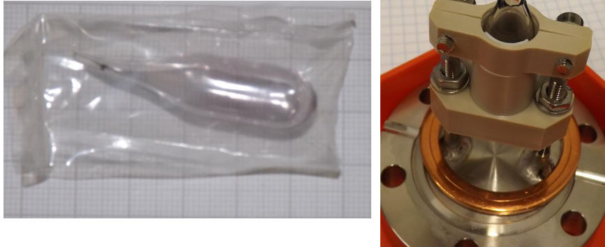
Figure 2.12 – Quartz ampule which was used for the irradiation of the enriched ^{36}\text{Ar} isotope mixture. The picture on the left hand side shows the quartz ampule after its irradiation. Due to safety reasons the ampule was put into a sealed plastic envelope before its irradiation. The paper in the background is a normal plotting paper as a size reference. The photograph on the right shows the remnants of the quartz ampule after its usage in the MainzTPC. The tail of the ampule is clear-cut while the body is still mounted to the ampule holder of the guillotine.
