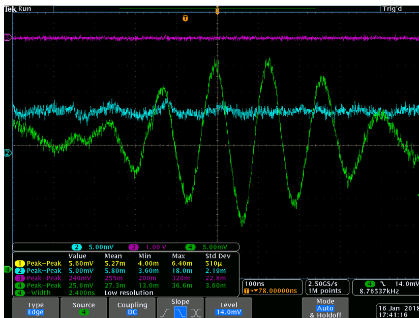
Figure 3.5 – Oscilloscope screenshot of the bipolar PTR noise. The green channels presents the signal output of the amplified top PMT.
