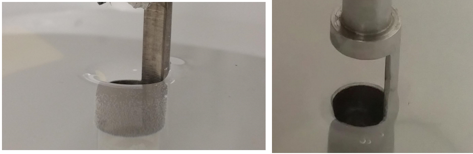
Figure 4.23 – Pictures of the liquid level tests with water. The old and new spillway are shown on the left and right hand side correspondingly. The picture on the left shows at the edge of the old spillway a pile-up of the liquid, while the new spillway in the picture on the right hand side does not. Both photographs were taken by David Maksimovic.
