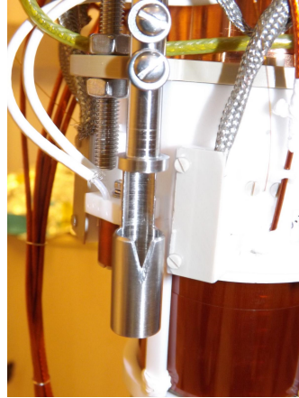
Figure 2.6 – Picture of the new spillway of the MainzTPC. Shown is the MainzTPC after its maintenance November 2017. The new spillway was designed by our Bachelor research assistant David Maksimovic and has compared to the old model a deep v-cut. Further all edges which are in contact with the LXe were sharpened in order to minimize the surface barrier the liquid has to overcome.
