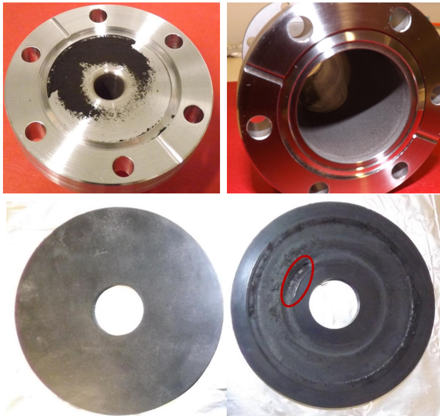
Figure 3.4 – Photographs of the black dust which was seceded from the inner diaphragm of the KNF double-diaphragm recirculation pump. The upper two pictures are showing the black dust which was found everywhere in the gas-system. The lower picture is a comparison of a new diaphragm with the old worn one. The red circle indicates the position where the worn diaphragm broke.
