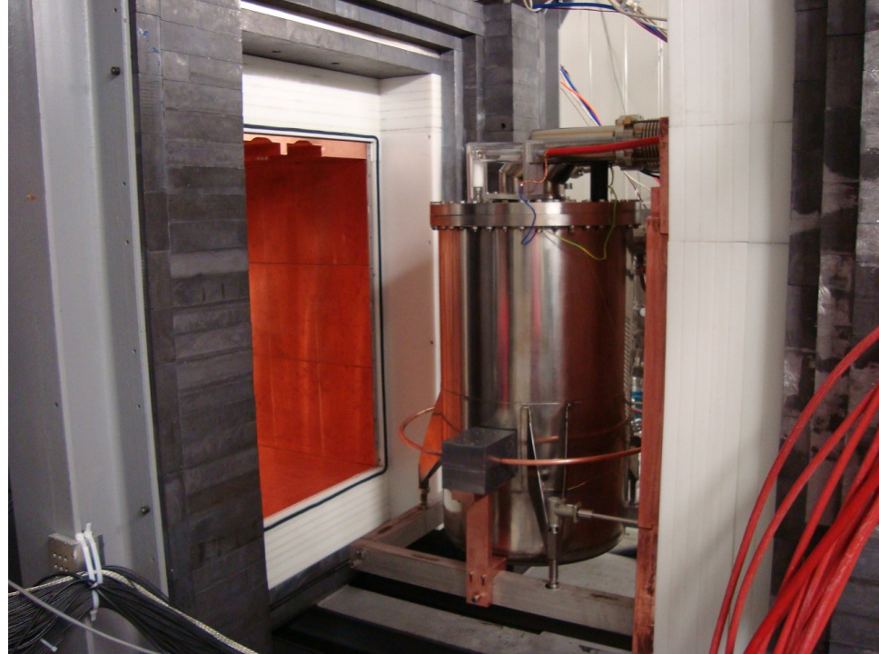
Figure 2.3: XENON100 Detector Structure and Passive Shield. A copper tube circling the detector is used to introduce calibration sources inside the passive shield and around the detector. The copper tube goes through a lead brick at one point. The ^{241}\text{AmBe} neutron source was placed at this point inside of the lead brick so that gamma radiation is suppressed.
