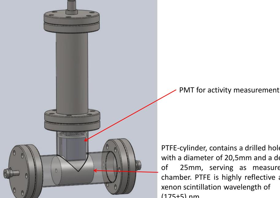
PTFE-cylinder, contains a drilled hole with a diameter of 20,5mm and a depth 25mm, serving as measurement chamber. PTFE is highly reflective at the xenon scintillation wavelength of (175±5) nm.
